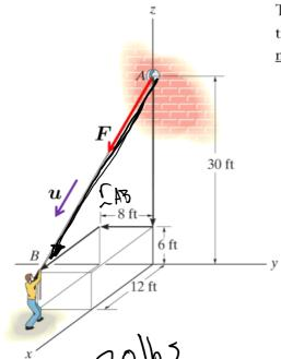
The force vector  $\mathbf{F}$  acting a long the rope can be defined by the unit vector  $\mathbf{u}$  (defined the <u>direction</u> of the rope) and the <u>magnitude</u> of the force.
